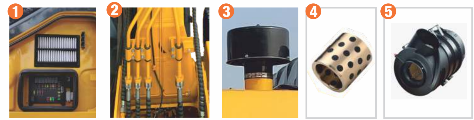
1. External accessibility to electric box 2. Flange type connectors 3. Air pre cleaner 4. Graphite bushes 5. Radial seal air filter
