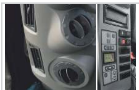
Automatic climate control 9 air cooling vents
