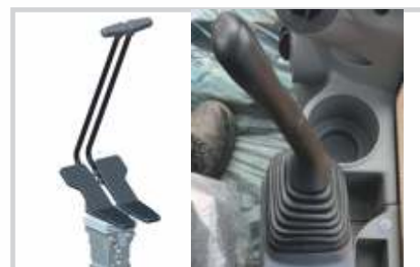
Smooth travel pedal and thin joystick provide excellent grips
