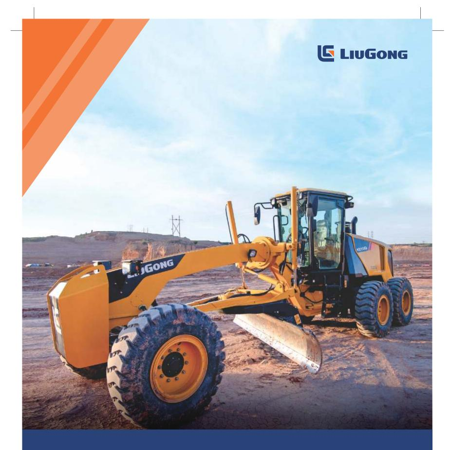
Engine Gross Power Std.Operating Weight Standard Blade Cabin YUCHAI 217 hp @ 2,200 rpm 16,400 kg 3,960 mm Air Conditioned
