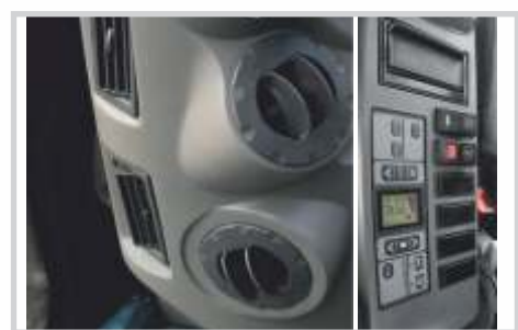
Automatic climate control 9 air cooling vents
